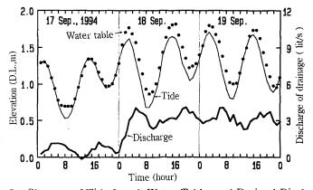
Figure 5 Changes of Tide Level, Water Table, and Drained Discharge. to the beach surface. In other words, the ground was completely saturated with the water. On the other hand, that in the drained beach which is denoted by circles was 0.6 meter lower in maximum than the beach surface. The area between the beach surface and the water table in the drained beach was unsaturated, which means that the groundwater was gathered to the permeable layer and drained offshore through the drainage pipe.
