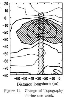
was steep in the area lower than 2m. In short, a new berm was formed on the foreshore above the permeable layer.
