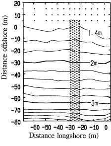
Figure 12 Foreshore Topography, after Erosion.
