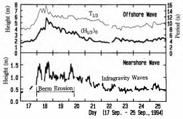
Figure 3 Waves in Typhoon No.9424.
