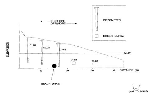
Figure 6. Cross-sectional schematic of the groundwater monitoring installation at Codfish Park STABEACH segment and adjacent control beach.
