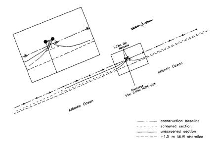
Figure 3. Plan-view schematic of Lighthouse North STABEACH segment.
