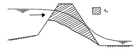
figure 6: definition of the eroded cross-section  $A_d$
