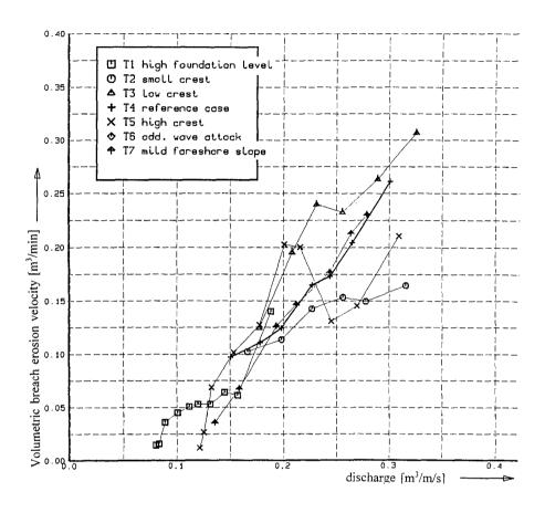
figure 7: volumetric breach erosion velocity as a function of the water discharge in the breach
