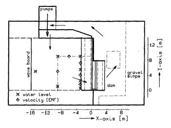
In order to complete this description of the experiment set-up, in figure 1 a planview of the wave basin lay-out is shown.
