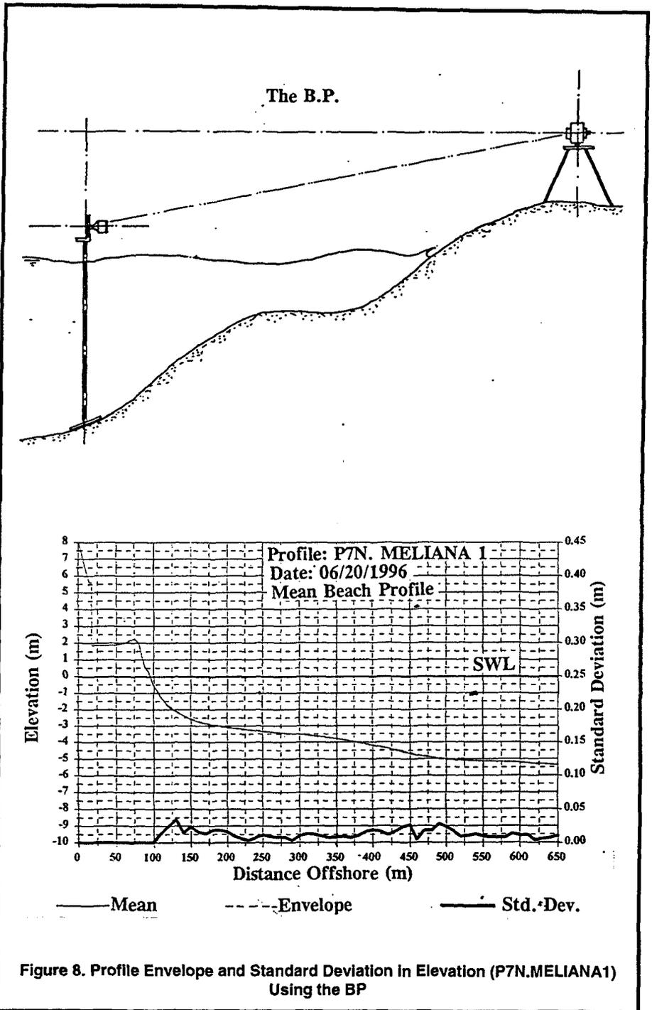
**Figure 8. Profile Envelope and Standard Deviation in Elevation (P7N.MELIANA1) Using the BP**
