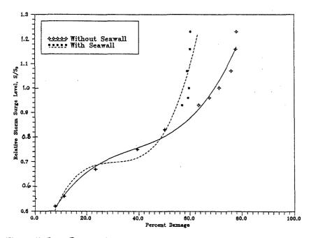
Figure 4b Dune Damage Curve: Percent Loss Versus  $S/S_D$
