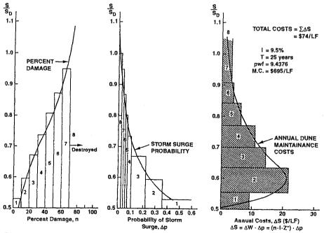
Figure 7 Probabilistic Design Method for Dune Maintenance Costs
