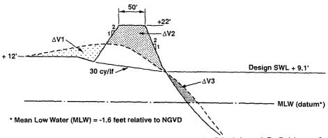
Figure 3 Dune Cross-Section Design for Dam Neck, Virginia and Definitions of Volume Change Regions,  $\Delta V1$ ,  $\Delta V2$  and  $\Delta V3$ .
