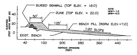
Figure 5 Dune-Beach-Buried Seawall Design for Dam Neck, VA
