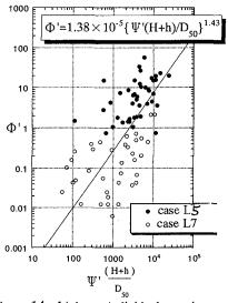
Figure 14.  $\Phi'$  due to individual uprush and  $\Psi'(H+h)/D_{s0}$
