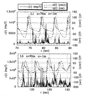
Figure 4. Fluctuation of suspended sand concentration due to wave motion in the case L1 and L6
