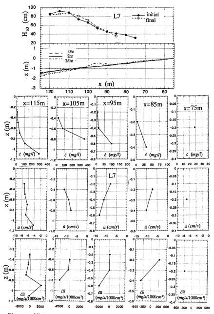
Figure 8. Virtical distribution of suspended sand transport flux in the case L7
