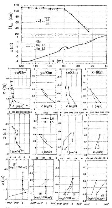
Figure 7. Virtical distribution of suspended sand transport flux in the cases L5 and L6
