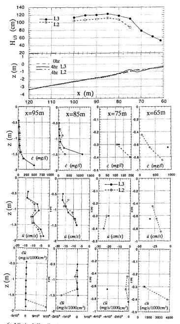
Figure 6. Virtical distribution of suspended sand transport flux in the cases L2 and L3
