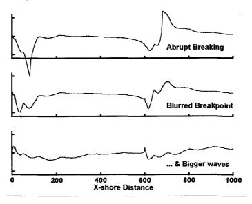
Figure 9(a) SFC for a band of long waves (0.01–0.04Hz), (b) inclusion of uncertain breaking & (c) bigger short waves.
