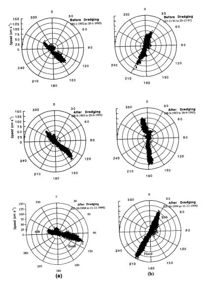
Fig. 6. Current velocities at 1 m above the bed before and after dredging at: (a) the edge of Cutter Channel and (b) at Lower Western Channel near Panepane Point.
