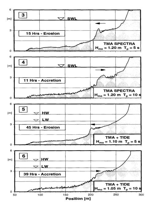
Figure 3. Initial and final beach profiles under spectral waves with constant water level (Test Series 3 and 4) and spectral waves with superimposed tidal simulation (Test Series 5 and 6)
