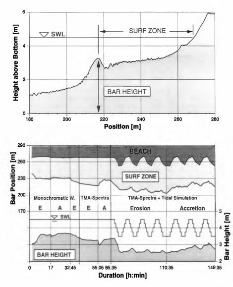
Figure 5. Definition of the surf zone (above) and position and height of bar over all Test Series' (below)
