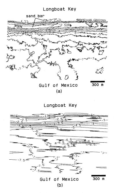
Figure 3.1 Longboat Key, Florida, November 1995: a) representative section of SHOALS bathymetry, b) simulated profile bathymetry at 300-m spacing. All depths are in meters referenced to NGVD.
