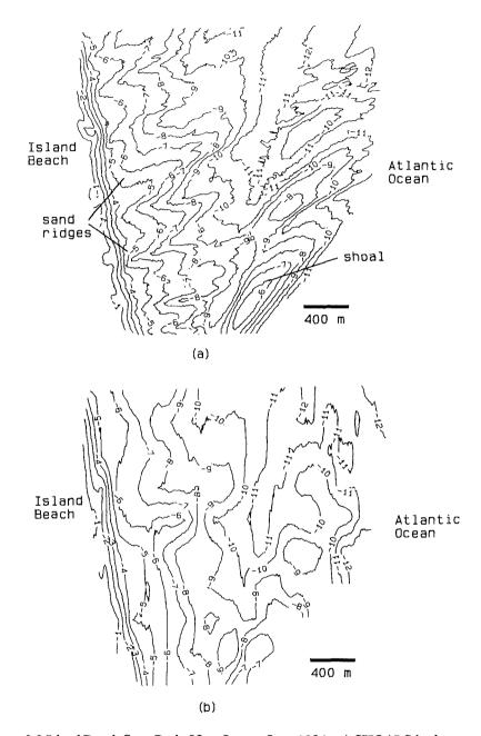
Figure 3.2 Island Beach State Park, New Jersey, June 1994: a) SHOALS bathymetry, b) simulated profile bathymetry at 300-m spacing. All depths are in meters referenced to NGVD.
