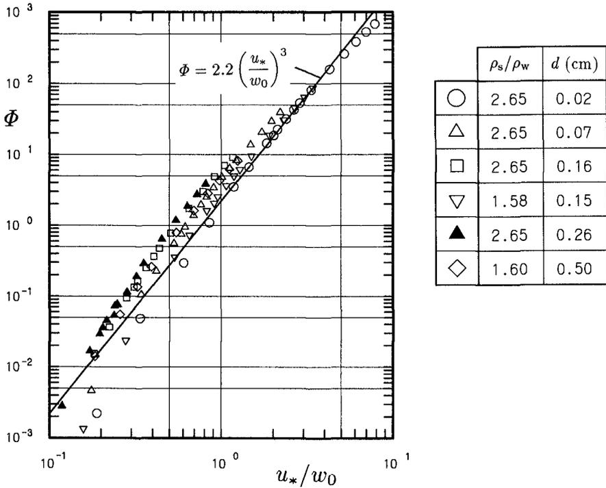
Fig. 4 Relation between  $\Phi_{cal}$  and  $u_*/w_0$  in sinusoidally oscillatory flow.
