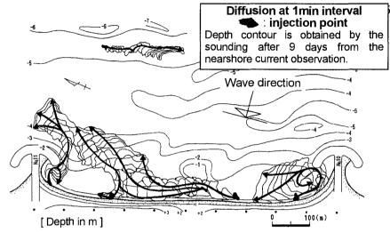
Fig.5 Diffusion of injected dyed water between No.10 and No.11 headlands( Dec. 7th, 1993 ).
