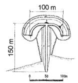
Fig.3 Plane shape of anchor-type headland.
