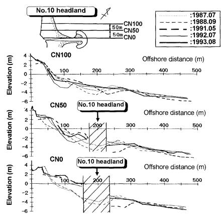
Fig.10 Typical profile changes in a period between July, 1987 and August, 1993.
