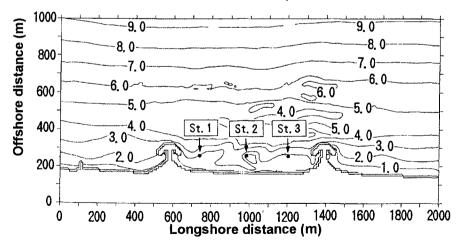
Fig.12 Original bathymetric chart ( Chart 1 ) and selected point for verification of wave direction.
