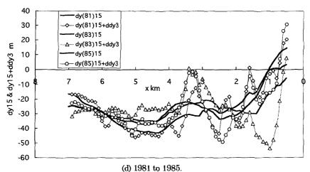
Figure 4. Total shoreline changes with erosive waves (W) down-coast from the river mouth.
