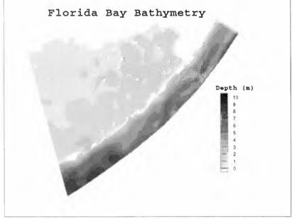
Figure 2. Bathymetry contours in the entire finer-grid model domain. All depths inside the Bay are less than 1-2 meters.
