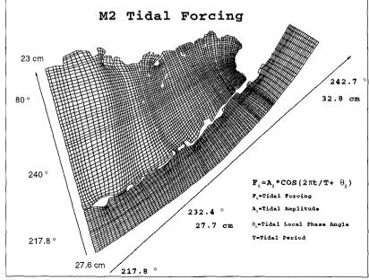
Figure 6. A model grid with 98x75 cells and open boundary conditions for  $M_2$  tide in Florida Bay.
