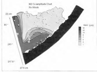
Figure 7. Co-amplitude chart of  $M_2$  tide simulated by the 3-D model.
