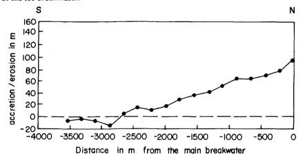
Figure 2. Difference in m between the mean position of the shoreline in 1958-1964 and that of 1983-1992 south of Ashdod Port.
