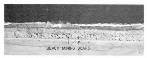
Figure 11. Aerial photograph taken in 1958 showing the scars of beach mining along the Ashdod shoreline.
