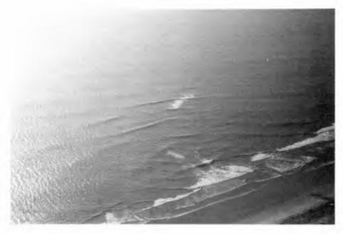
Photo 1. Wave Refraction due to Nearshore Berm. 12/92.
