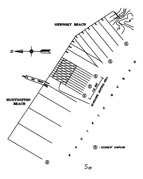
Figure 1. Monitoring Program Schematic.
