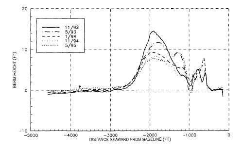
Figure 3. Comparison of Profile Differences at Line 19 Relative to Pre-project Condition (12/91).
