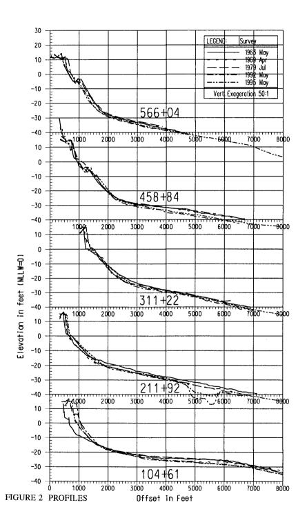
values estimated from formulae and wave statistics, ie. the 12-hour annual wave at Huntington Beach of 233 cm based on four years of observation results in a computed depth of closure of 16 feet (Hallermeir, 1981). It also does not have to assume a priori insignificant sediment transport across the boundary.
