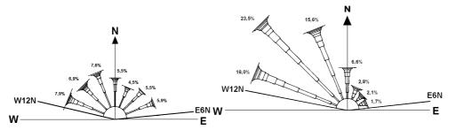
Figure 5.Joint distribution visual wave height / direction, distinguishing between types of waves Sea (left) and Swell (right).
