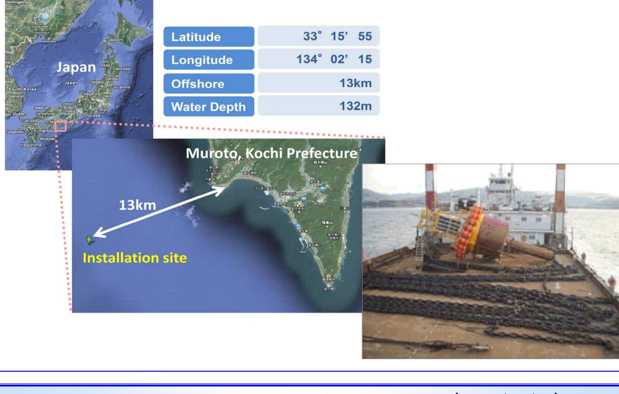
Mooring system of the GPS buoy needs to be designed to follow the wave actions as much as possible, in order to obtain more exact ocean wave and tsunami data.
