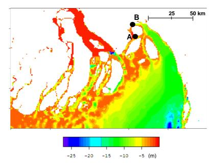
Figure 3. Bathymetry of the Meghna Estuary after correcting unrealistic water depth of GEBCO data and updating the coastlines using satellite images.
