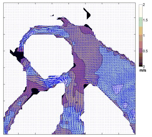
Figure 7. Simulated tidal velocity distribution during peak flood velocity at the measurement location B, contour shows velocity magnitude in m/s
