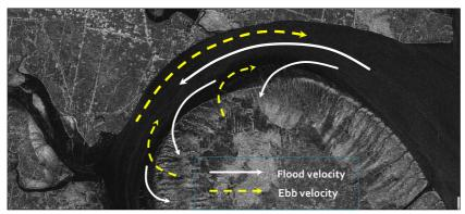
Figure 10. Tidal current features around the study site
