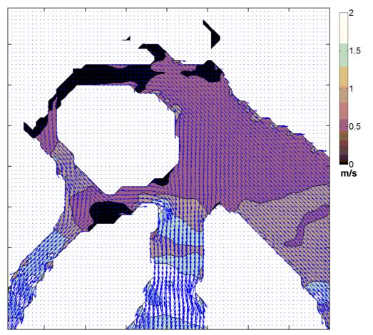
Figure 8. Simulated tidal velocity distribution during slack before ebb (SBE) at the measurement location B, along with contour of velocity magnitude (m/s)
