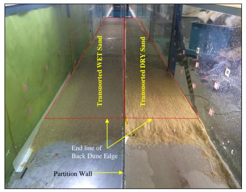
Figure 5. Transported sediment collection area (marked by red box) on the flume bed
