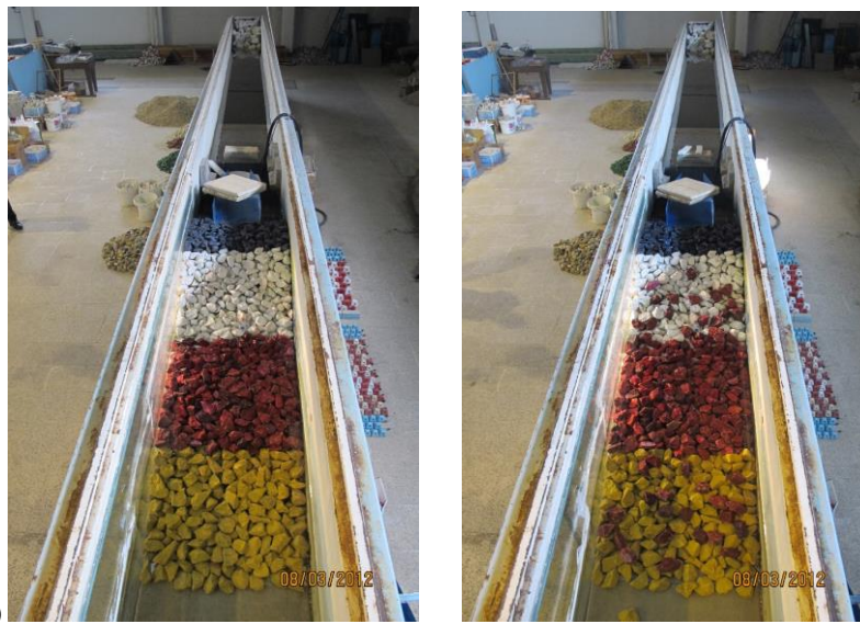
Figure A.12 (a) Before, (b) After the experiment wave set for the Second Cross Section– Alternative 4
