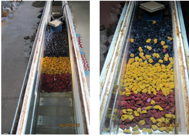
Figure A.11 (a) Before, (b) After the experiment wave set for the Second Cross Section – Alternative 3
