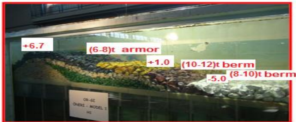
Figure 15 View of the Second CrossSection breakwater model in the wave channel
