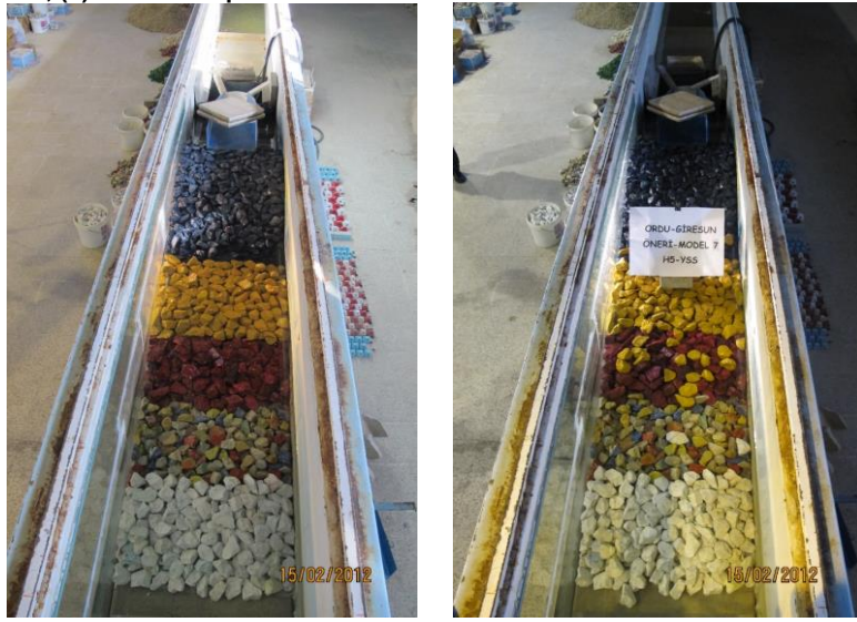
Figure A.10 (a) Before, (b) After the experiment wave set for the Second Cross Section – Alternative 2
