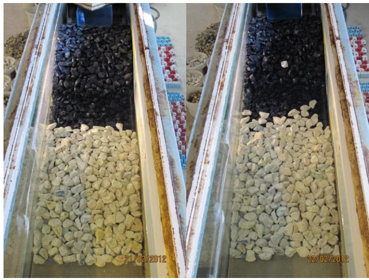
Figure A.4 (a) Before, (b) After the experiment wave set for the First Cross Section – Alternative 2
