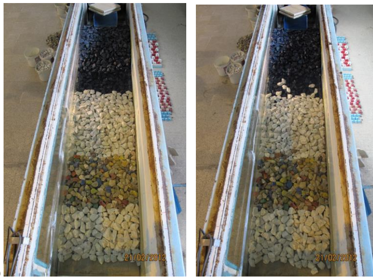
Figure A.3 (a) Before, (b) After the experiment wave set for the First Cross Section – Alternative 1
