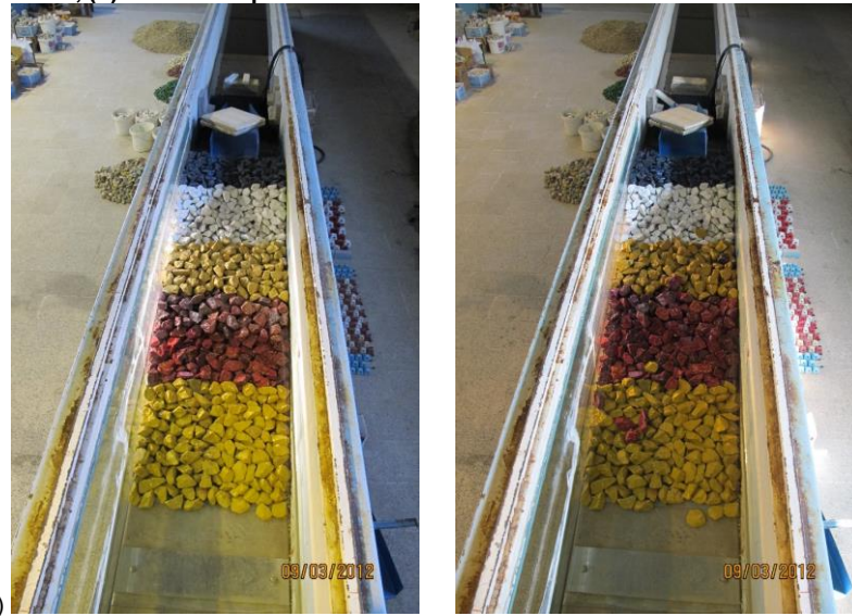
Figure A.13 (a) Before, (b) After the experiment wave set for the Second Cross Section – Alternative 5
