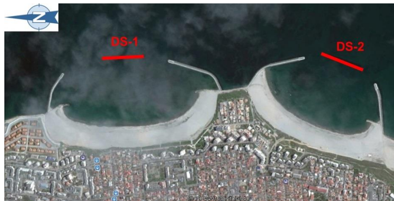
Figure 2 Location of the submerged breakwaters within the coastal protection system (DS-1 in Tomis North area and DS-2 in Tomis Centre area)
