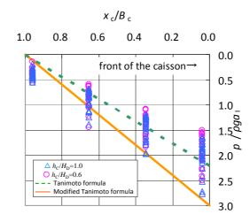
Figure 11. Non-dimensional uplift pressure distributions.
