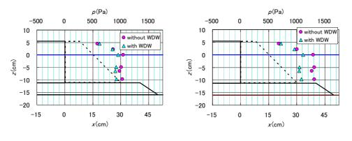
(a) Non-breaking (b) Breaking Figure 8. Examples of instantaneous wave pressure distribution. (Case 1-1)
