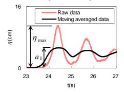
Figure 6. Definition of Incident Tsunami Height.
