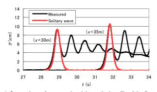
Figure 4. Comparison of measured and theoretical profile of the first soliton.
