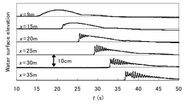
Figure 2. Time historical profiles of tsunami. (*h*=10cm, *T*=22s)
