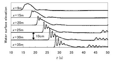
Figure 3. Time historical profiles of tsunami. (h=28cm, T=12s)
