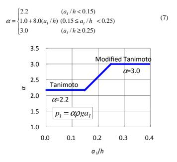
Figure 12. Proposed horizontal wave pressure coefficients  $\alpha$
