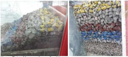
b) Photos of the composite seawall model Figure 2 Cross-section of a composite seawall model
