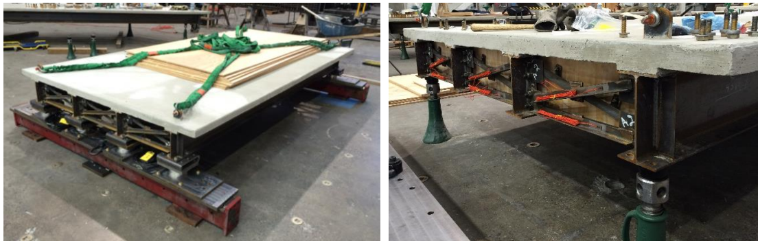
Figure 2. I-girder composite bridge with cross-frames (left) and attached plywood diaphragms (right) during the assembly in the Large Scale Structures Lab at the University of Nevada, Reno
