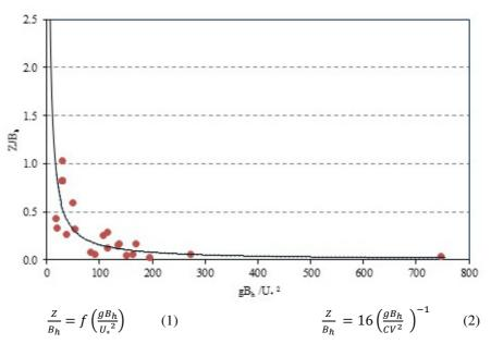
Figure 7. Relationship between representatives scour depth and shear velocity for surveyed locations in NE Japan.
