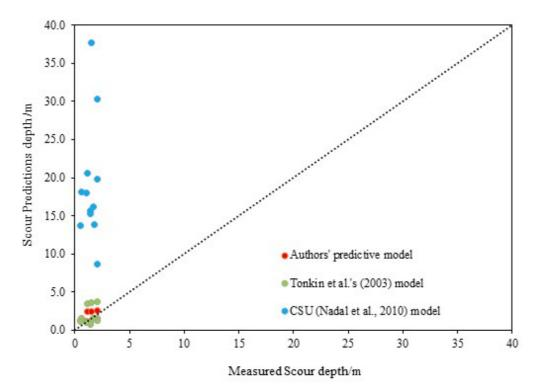
Figure 8. Comparison results of all three predictive models against the measured field data.
