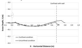
Figure 2 - Scour profile on sand bed ( $d_{50}$ =0.52 mm) with a quay wall at X<sub>w</sub>=0.7m distance from the face of propeller at equilibrium stage (G=0.1m, D<sub>p</sub>=0.65 m, 745 rpm)
