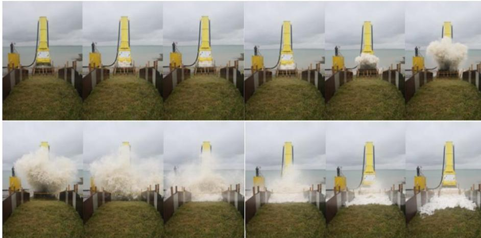
**Figure 10. Impression of wave impact on step.**
