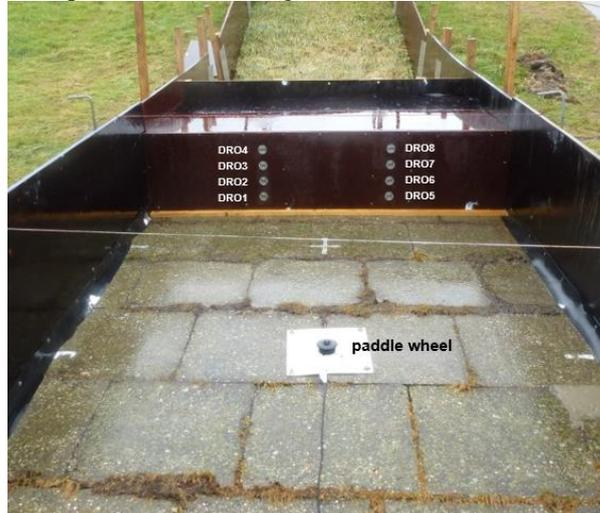
**Figure 9. Pressure sensors in the step.**
