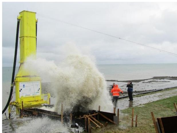
**Figure 7. Wave impulse with the wave run-up simulator**
