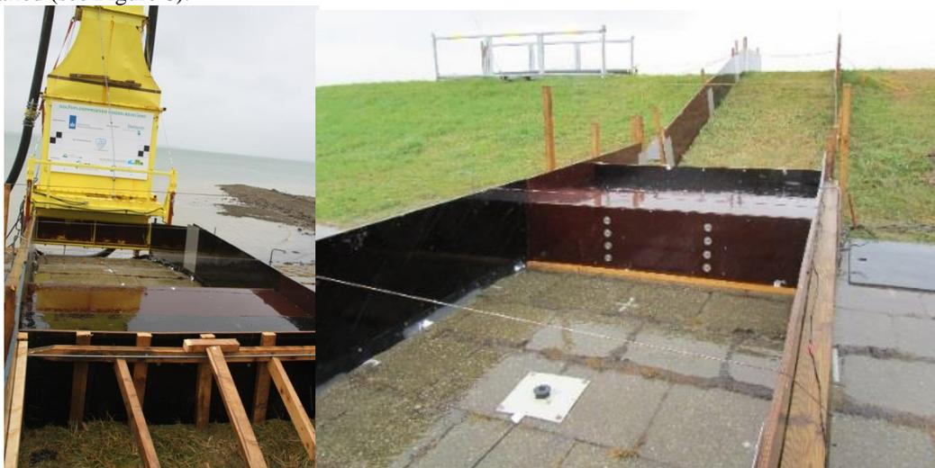
**Figure 8. Overview wave run-up simulator and the first step with 8 pressure transducers.**
