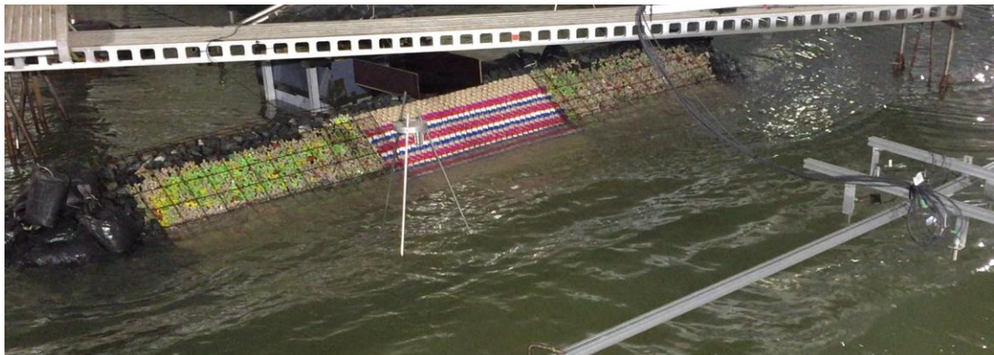
Figure 5: Breakwater model in 3D tests (front view)
