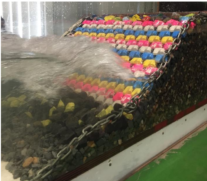
Figure 2: XblocPlus armoured 3:4 breakwater slope in the DMC wave flume
