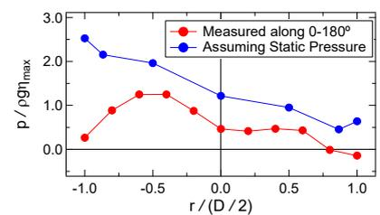
Figure 4 Pressure on Bottom of Tank
