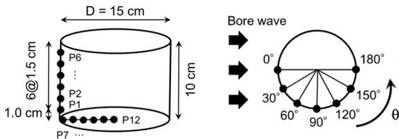
Figure 1 Pressure Measuring Points on Cylindrical Tank
