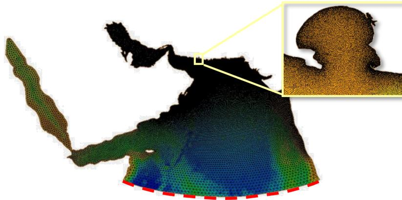
Figure 7. Computational grid of wave and ocean models
