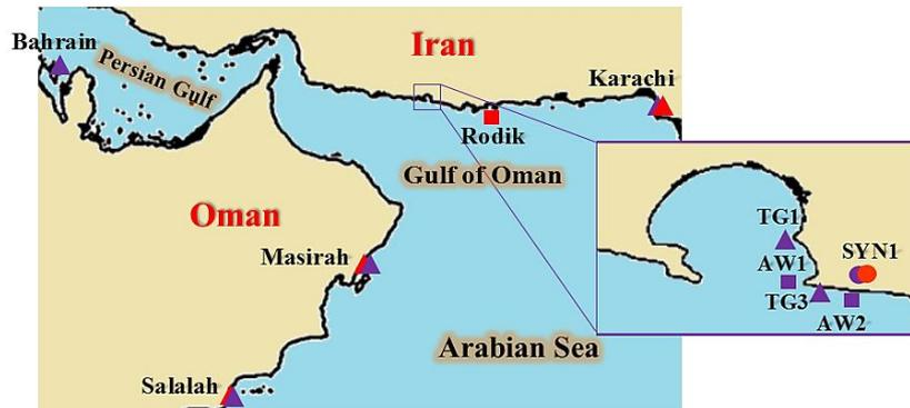
Figure 1. Wind stations (circle), ADCPs (square), tide gauges (triangular) during cyclone Gonu (violet) and Ashobaa (red)
