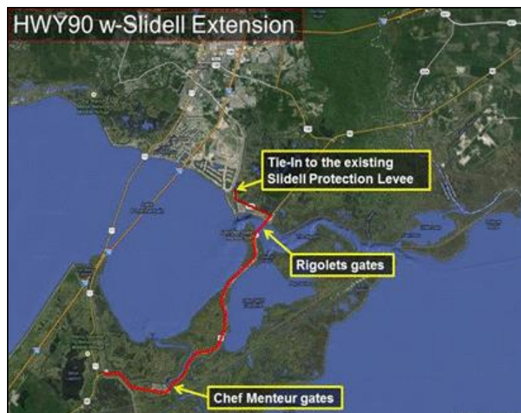
Figure 7. Map of potential Highway 90 LPB alignment with ties to existing New Orleans and Slidell levees.
