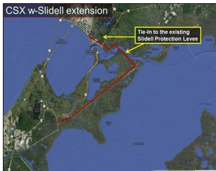
Figure 8. Map of potential CSX railway LPB alignment with ties to existing New Orleans and Slidell levees.
