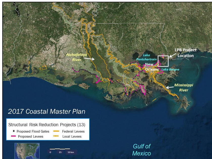
Figure 3. Existing and proposed structural risk reduction projects including planned Lake Pontchartrain Barrier.
