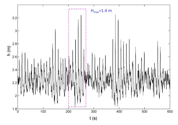
$h_0=2.25 \text{ m}, H_s=0.70 \text{ m}, T_p=11.1 \text{ s}$
