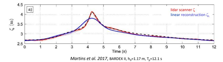
$\rightarrow$  provides a poor description of the peaky and skewed shape of nonlinear waves  $\rightarrow$  underestimates the individual wave height by up to 30 %
