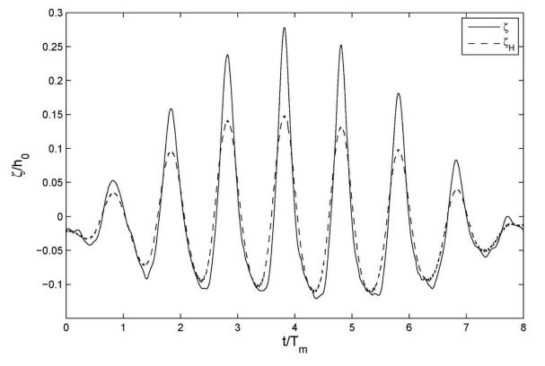
$\zeta$  and P<sub>m</sub> were synchronously measured in the shoaling zone, at 18.5m from the wave maker; h<sub>0</sub>=0.326 m, T<sub>m</sub>=1.7 s, µ=0.53
