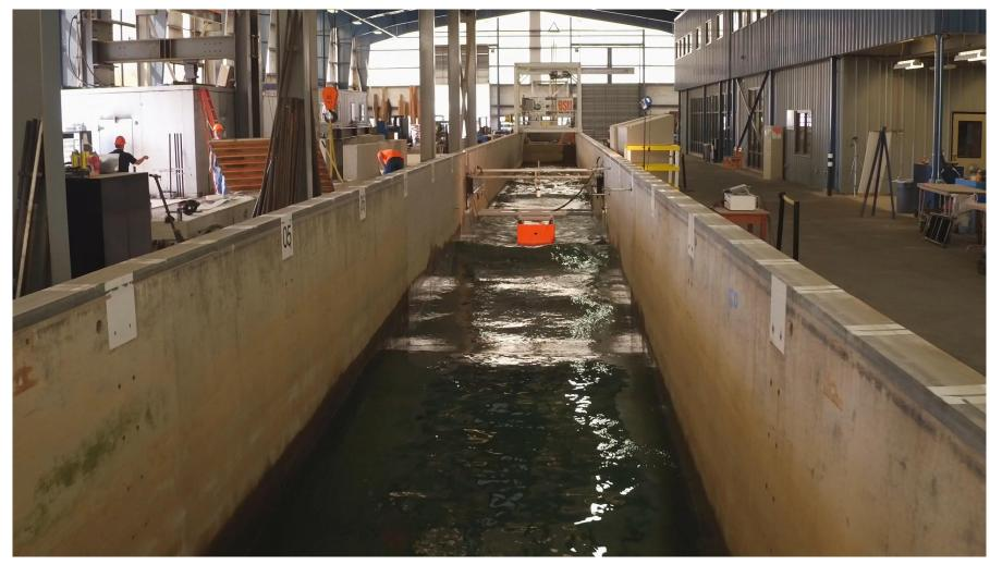
Characterize horizontal and vertical wave-induced pressures and loads on elevated structures for various wave/surge conditions
