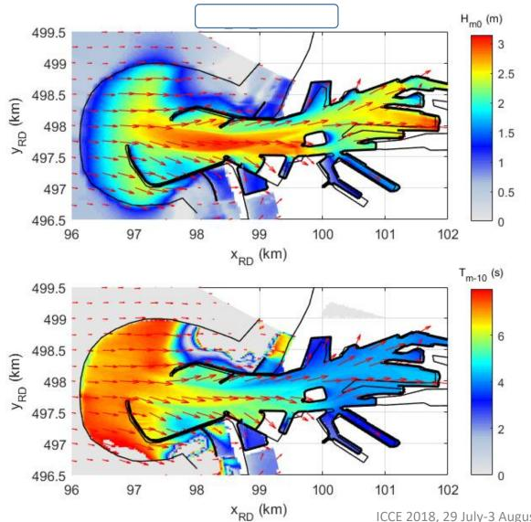
Wave growth  $E_G$  on top of penetrated wave field in PHAROS domain
