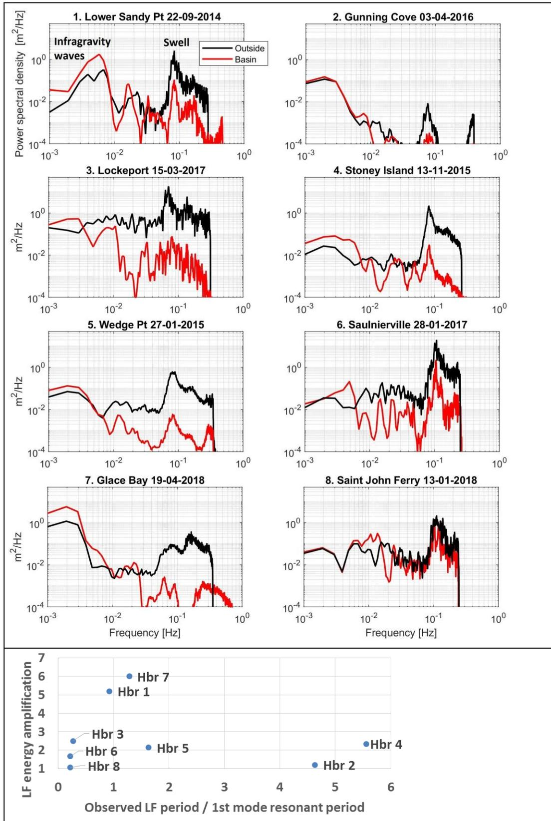
Figure 4. Top 8 plots: Frequency analysis of harbour wave gauge observations – Bottom plot: LF energy amplification vs. closeness of observed LF period to first mode resonant period estimated from analytical tools. The results show resonance is caused by incident LF wave energy coinciding with natural resonant period of the basin, particularly for Harbours 1 and 7.
