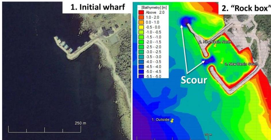
Figure 2. Harbour 1 layout and formation of long wave-induced scour holes, with three wave gauge locations
