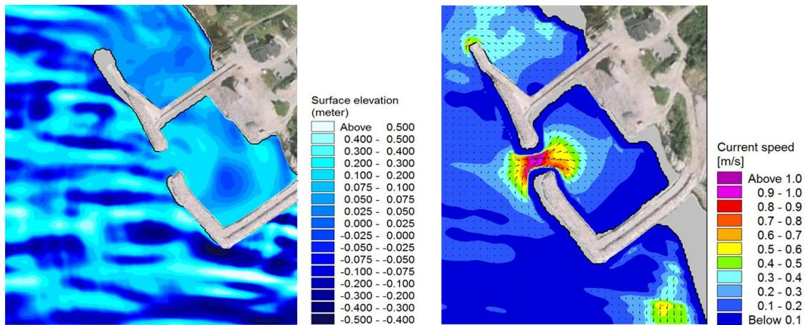
**Figure 5. Sample modeled sea surface elevation (left) and long-wave induced resonance currents (right) at Harbour 1**
