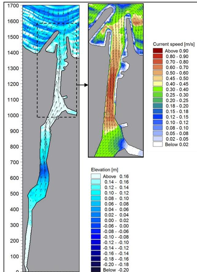
Figure 8. Phase Resolving Wave Model Snapshot (left) and Associated Currents (right)
