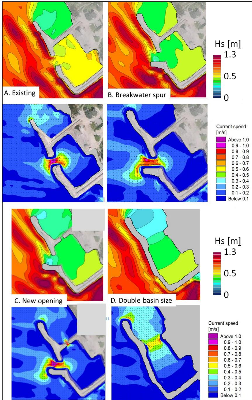
Figure 6. Sample modeled Hs (including swells + resonance) and resonance currents (right) at Harbour 1 for various basin reconfiguration options
