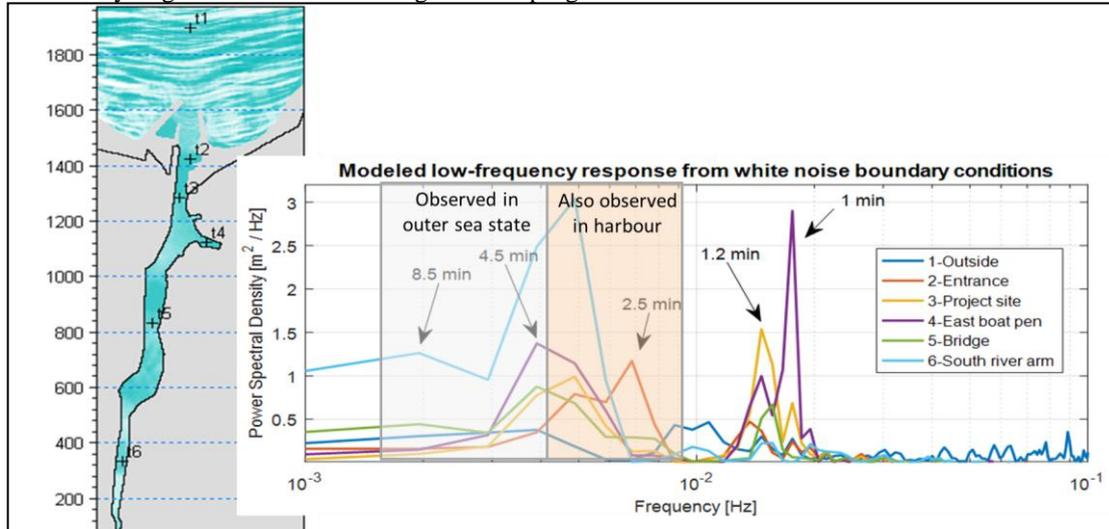
Figure 7. Results of White Noise Simulation with BW Model, Showing Natural Oscillation Frequencies
