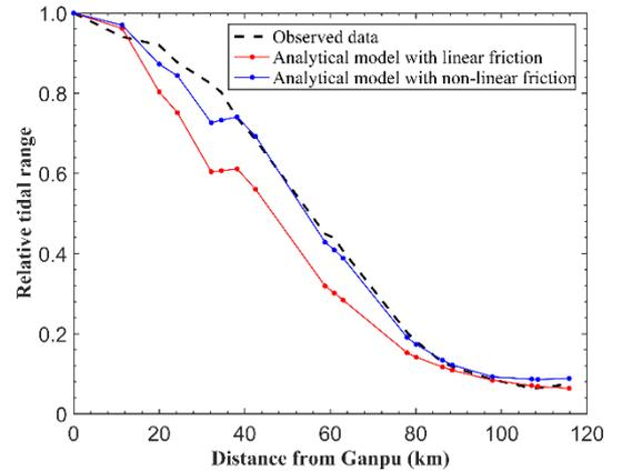
Figure 1 Comparison of linear and non-linear friction model results with observations
