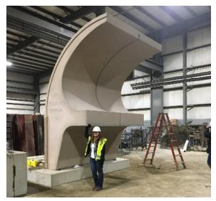
Figure 1 - Precast Individual Wall Sections
