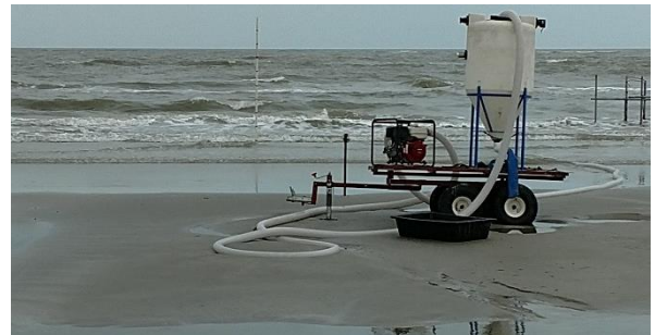
Figure 2 - Scale Model Sampling Equipment for Sediment Bypassing/Back-passing System.
