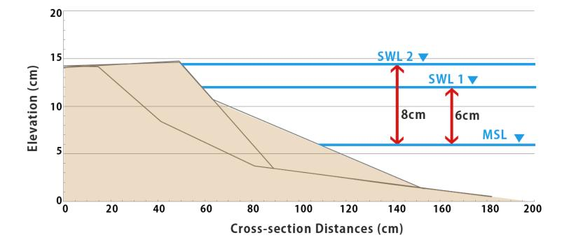
Two water levels (SWL1 and SWL2) above the mean sea level (MSL) of 6 and 8 cm because of the sensitivity of erosion and flooding risk to the water level
