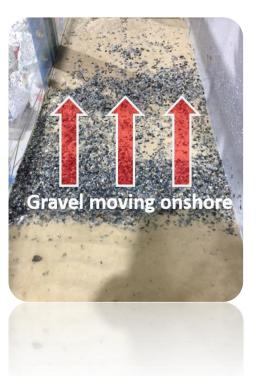
Sand : d<sub>50</sub> = 0.16mm, density=2.50g/cm<sup>3</sup> Gravel : d<sub>50</sub> = 5.00mm, density=2.68 g/cm<sup>3</sup>
