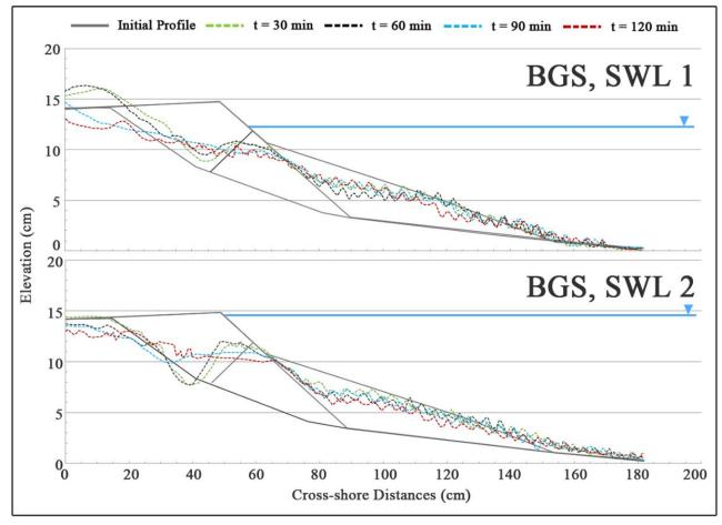
The sill's effect became noticeable only after the sill's crest was exposed but wave breaking over the exposed crest created a scour hole landward of the sill
