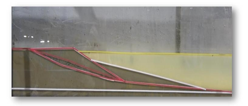
Buried gravel layer may prevent lowering of eroded sand berm and facilitate an equilibrium profile development
