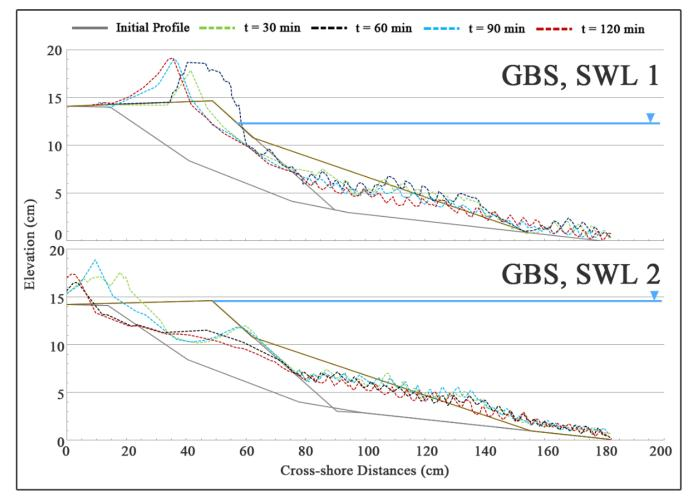
Gravel deposition and landward migration were sensitive to SWL because wave runup on gravel is sensitive to SWL
