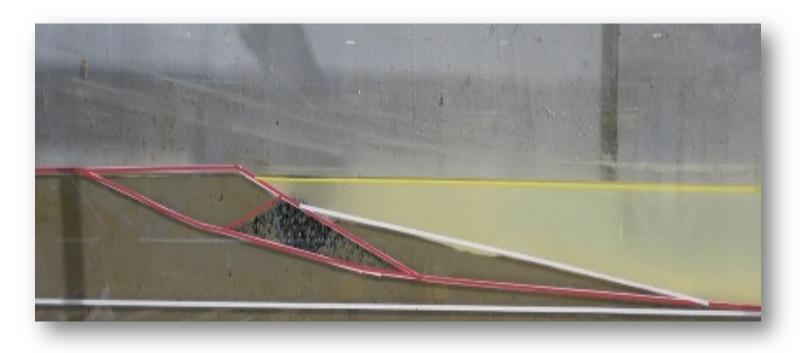
• Buried gravel sill may reduce the extent of berm erosion and does not spoil shore aesthetics
