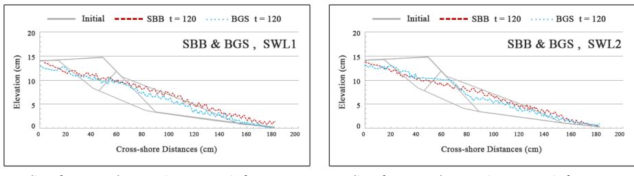
2 lines for SBB and BGS at time = 120 min for SWL 1
