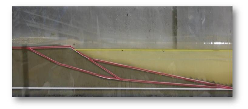
• Berm slope of 1/3.5 and beach slope of 1/11
