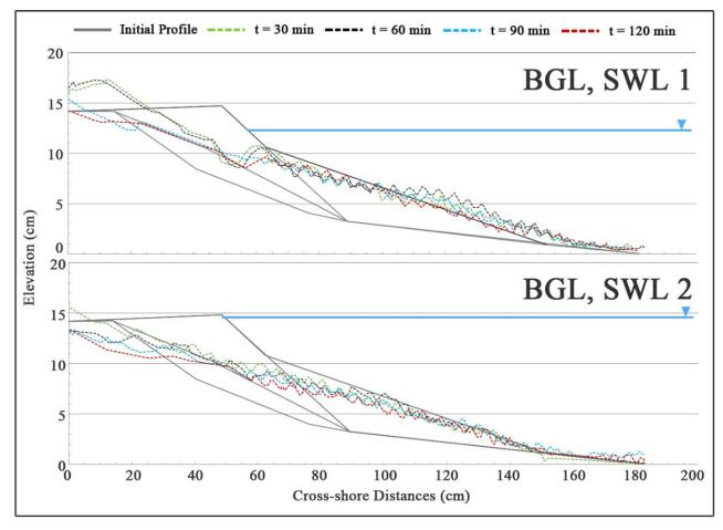
The landward edge of the gravel layer was eroded after the berm erosion progressed landward and the thin layer of gravel did not protect sand below the gravel layer
