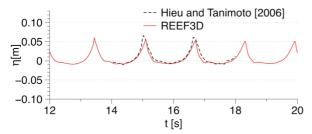
Figure 4 - Free surface elevation at WG4 over the toe of the leeward slope of the submerged breakwater
