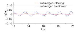
Figure 9 - Free surface elevation at WG8, a location just behind the floating breakwater, with and without the floating breakwater on the lee side.
