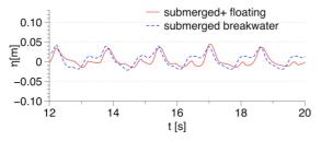
Figure 7 - Free surface elevation at WG6 at about L/2 from the toe of the leeward slope of the submerged breakwater, with and without the floating breakwater on the lee side.
