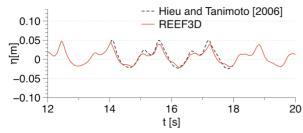
Figure 5 - Free surface elevation at WG6 at about L/2 from the toe of the leeward slope of the submerged breakwater
