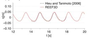
Figure 2 - Free surface elevation at WG1, upstream of the porous submerged breakwater showing the incident waves
