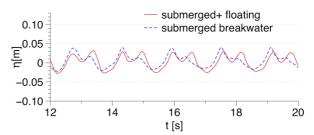
Figure 8 - Free surface elevation at WG7, a location just in front of the floating breakwater, with and without the floating breakwater on the lee side.
