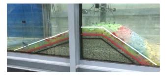
Figure 2.Lateral view of rubble-mound breakwater without crown wall
