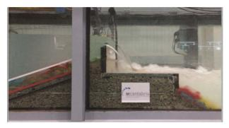
Figure 1. Overtopping over RMB with crown wall.
