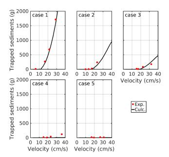
Figure 3 - Trapped sediments mainly due to bed load transport in the flume experiment (red dot) and the numerical simulation (black line) under unidirectional flow conditions.
