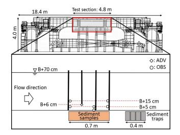
Figure 2 - Instrumentation layout in the flume.
