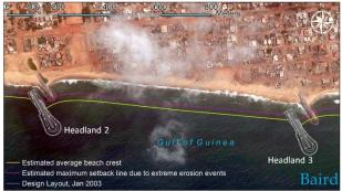
Figure 3 - Design vs. constructed Headlands 2 and 3 locations. The shoreline eroded approximately 100 m between completion of design and start of construction
