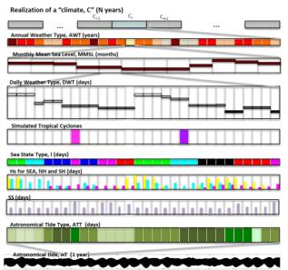
Figure 1 – Conceptual layout for downscaling climate to chronological oceanic and atmospheric conditions affecting TWLs.
