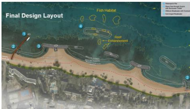
Figure 2. Design rendering for beach stabilization showing submerged breakwaters and enhancement structures.
