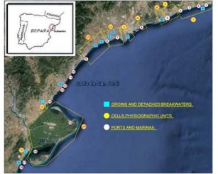
Figure 1 - Location of cells, ports an marinas, and protection beach works
