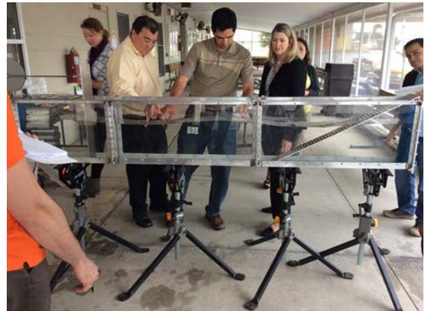
Figure 2. A portable wave flume being used by participants during a 3-day professional training course.
