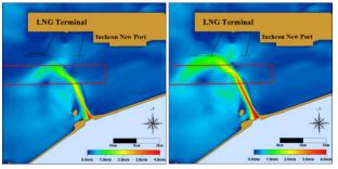
Figure 2 Numerical Simulation results (Left: discharge 5,000m<sup>3</sup>/sec, Right: discharge 8,000 m<sup>3</sup>/sec)
